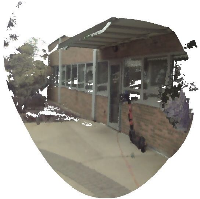
Fig. 8: Point cloud colored with corresponding RGB values to show qualitative results of calibration.
